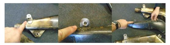
The small bracket with two screws on is for fitting the front part of the heatshield on-
