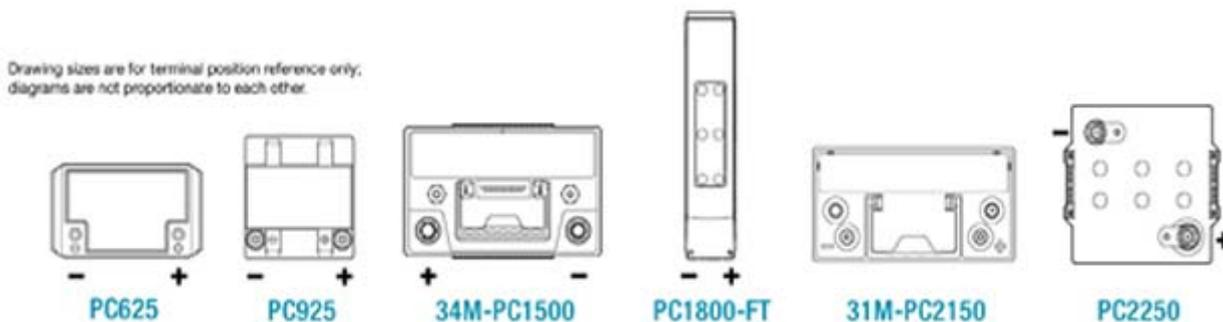
Drawing sizes are for terminal position reference only; diagrams are not proportionate to each other.
