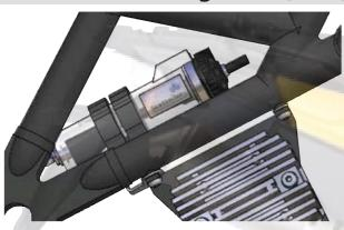
1. Unbolt and remove the regulator rectifier from the frame using a T30 Torx wrench.
