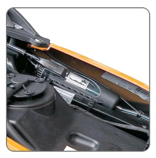
Shown above is the location for the oil reservoir (RMV), showing it attached to the outside of the left hand seat rail on the subframe. BMW supply a bracket with the TRA00002 kit, but it isn't required for the F800R. It's included as the kit is the same for both R and GS models. You can also mount a Lube Tube if you wish, see below;
