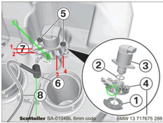
The BMW F800R (USA) has **5** intakes; the fifth is to connect the EVAP anti-polluting system, as shown in the image on the right.
