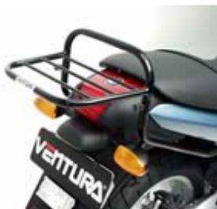
The Sports-Rack is designed for around town use and is interchangeable with the Pack-Rack in seconds. It also doubles as a grab handle for the passenger.
