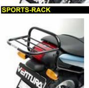
The Sports-Rack is designed for around town use and is interchangeable with the Pack-Rack in seconds. It also doubles as a grab handle for the passenger.
