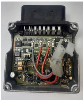
As you can see, this is a potentially fragile and exposed circuit board and it is important to make sure this doesn't get damaged as it can be a difficult to source part. It is also important to make sure it is sealed when fitting to the unit BRA90000. We suggest the use of silicone / instant gasket along the edge of the ECU and bracket to keep the electric circuit board sealed from water and dirt ingress. Attach ECU to the end of the bracket using the screws provided:
