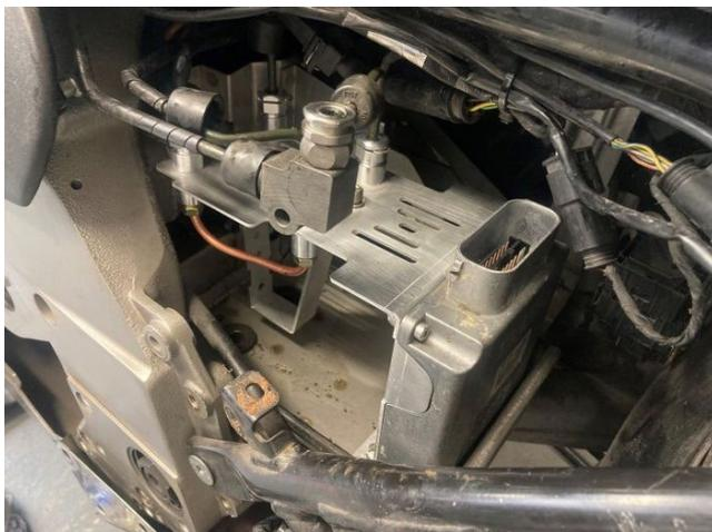
O-Rings are already installed in the top pipe connectors! Once the system is bled, you will be good to go, remembering that you have “conventional” braking, e.g. No ABS or linked brakes!
