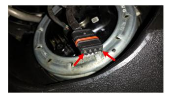
This must be 12 volts immediately after switching on the contact, after 20 sec. the voltage drops out again.
