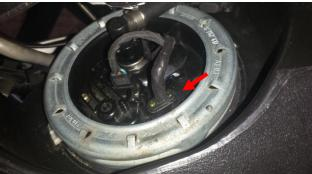
**Step 3:** Place on the disconnected connector in the fuel ribbon emulator.
