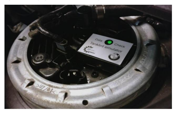
**Step 5:** Turn on the ignition and after 5 seconds the green LED "Data Check" lits up and gets voltage from the board computer.
