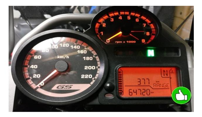
Once this fuel ribbon emulator has been installed, it is necessary to drive on the trip meter TRIP1 or TRIP2, as the tank indicator always shows a maximum.
