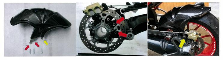
Please look for enough free clearance to all surrounding, and moveable components. Please mount all screws, and watch for the correct fitment of the parts, before tightening the screws. Please pay attention to the original torques (tightness's).
