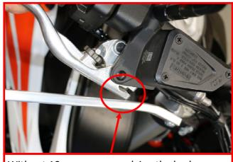
Without 10mm spacer applying the brake may cause lever to contact alloy backbone
