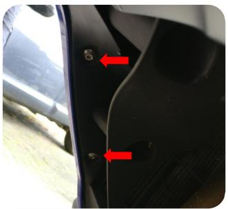
3. Disassemble the emblem bracket with the 2 torx screws on the inside of the fairing part.
