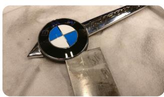
6. Remove the remaining tape from the back of the emblem and the R1200/1250RT bracket
