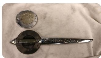
7. Drill an 8 mm hole in the center as shown. Through the chrome and black plastic at the rear.
