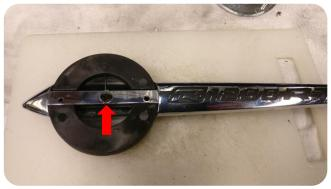
8. Degrease the place where the led indicator will be using the supplied alcohol pads and place them on the place of the original emblem.
