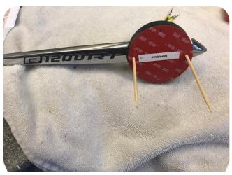
Remove the red protective tape on the back of the LED emblem indicator. Now press the led indicator firmly in place and remove the wooden pegs.
