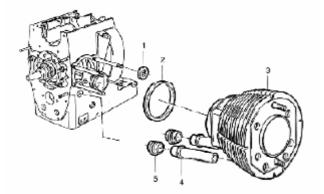
Push the pushrod rubber seals (nr. 5) on the pushrod protection tubes. Make sure the marking on the rubber is pointing outwards perpendicular to ground. Attention only for models from 9/80 on! Set the large O-ring (nr. 2) in to the groove on the cylinder foot.
