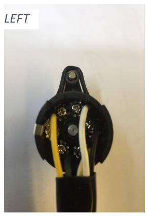
**ELA51220** With the switch in the central position work clockwise from the switch round the terminals using the following colours:
