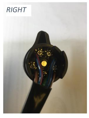
**ELA51219** NOTE: This switch must be wired to the end of the harness with the brake light switch spur (i.e the sub-harness with the green/black and green/red wires)
