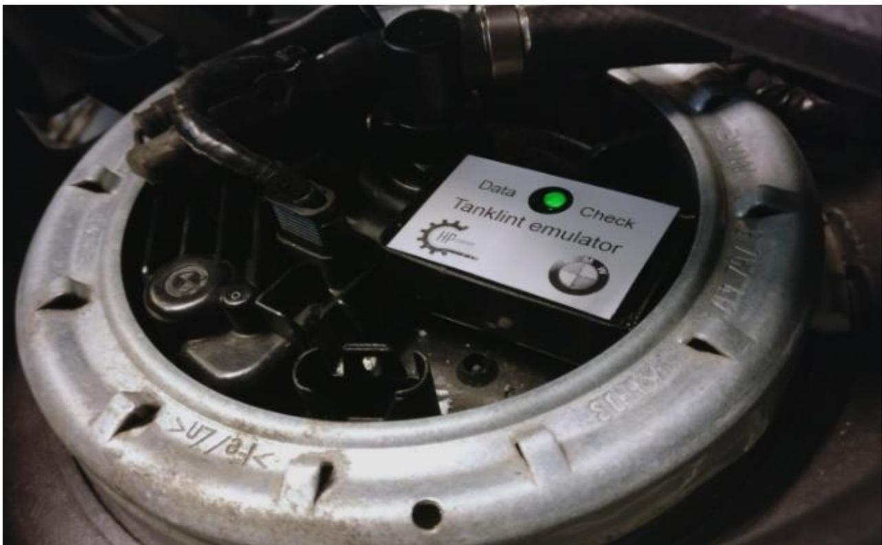
**Step 5:** Turn on the ignition and after 5 seconds the green LED "Data Check" lits up and gets voltage from the board computer.
